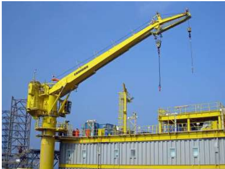
Pedestal fixed boom crane
