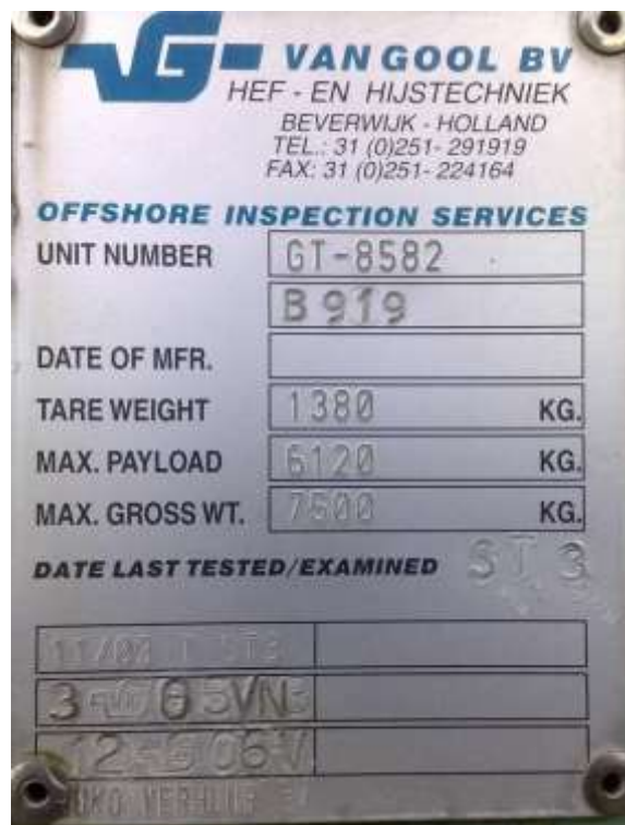
The most important data on the container, including the inspection details are shown on the inspection plate.
