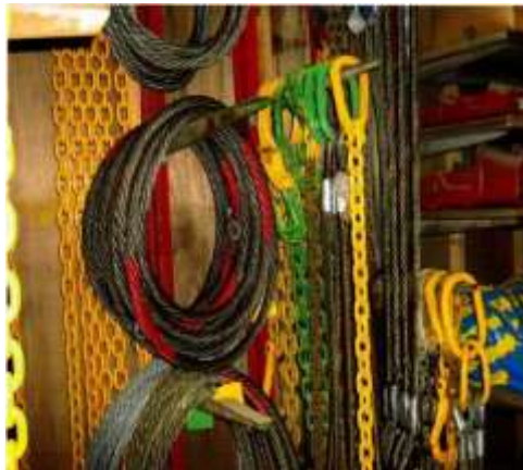
Storage of lifting tools
