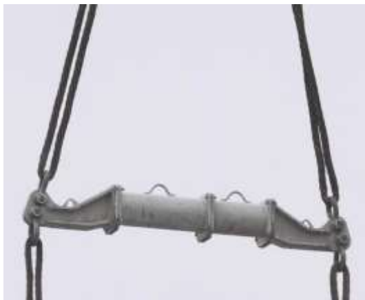
A lifting beam, spreader or leveller.
