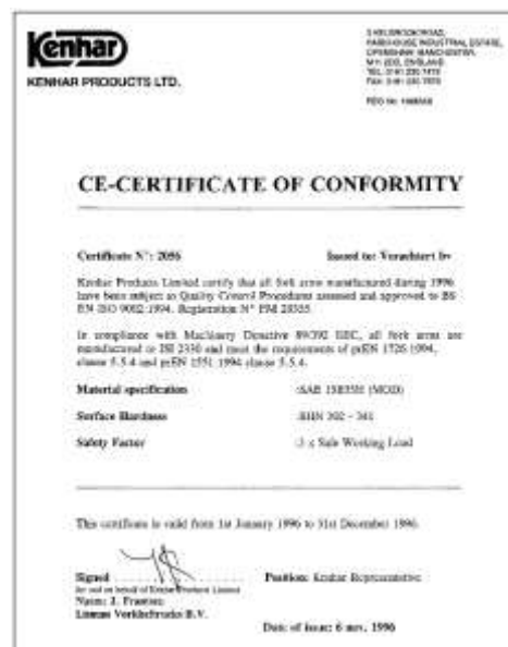
The Declaration of conformity must be present whit lifting equipment.
