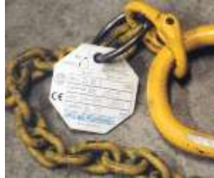
On lifting, tools must be a CE mark
