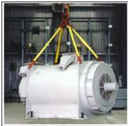
A four-leg fabric sling, made up of two round endless slings, connecting links, hooks and a master link.
