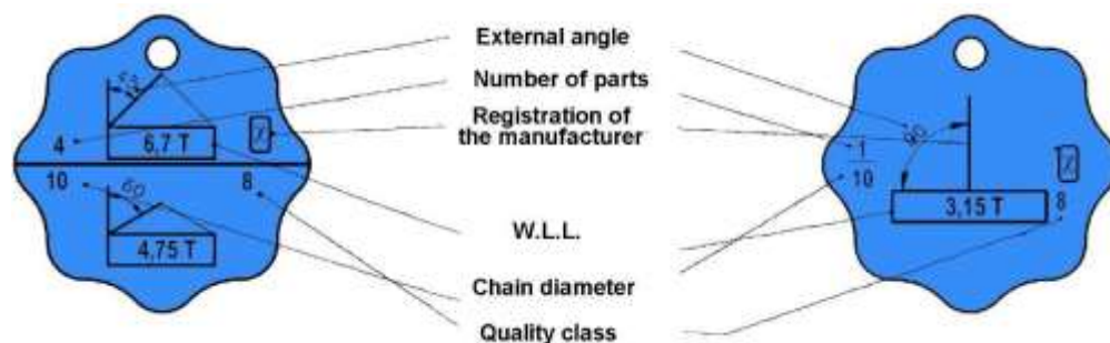
Type plate (tag-plate) for lifting tools.
